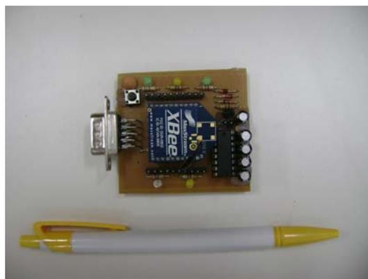
FIGURA 13 – Placa de Interface RS-232.
